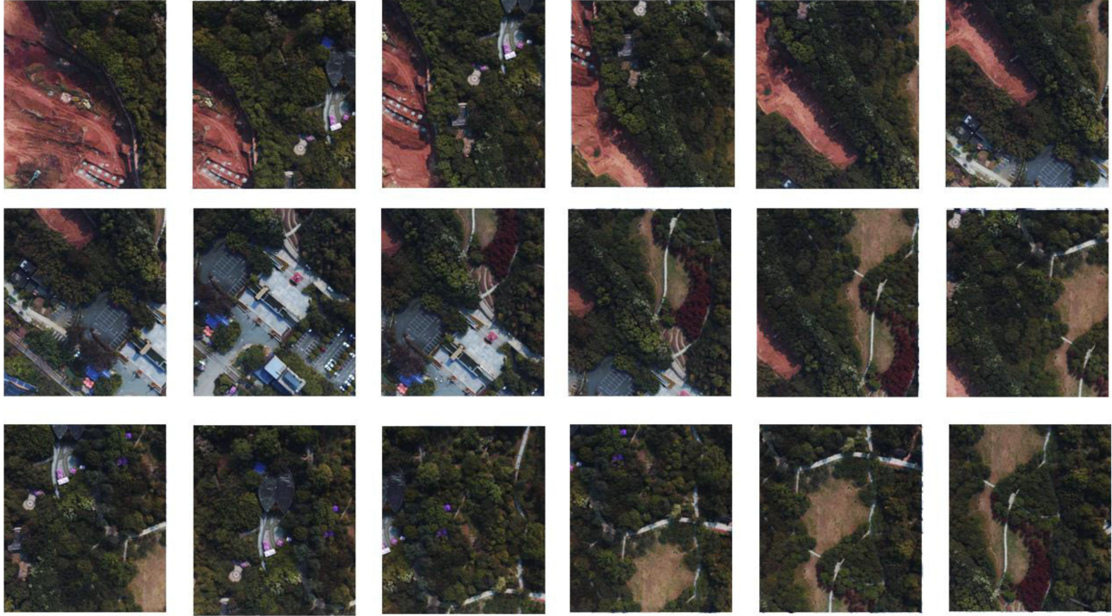
Fig. 2. Scenes for stitching were gathered by GaiaSky-mini sensor provided by SiChuan Dualix Spectral Imaging Technology Company, Ltd., which is a UAV-borne hyperspectral sensor whose wavelength ranges from 400 to 1000 nm. We synthesize the pseudocolor image by selecting the 92th (700.2 nm), 47th (547.6 nm), and 13th (436.5 nm) bands.
