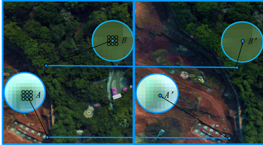
Fig. 8. Point A and its surrounding points in I_1 and point A' in I_2 , and point B and its surrounding points in I_1 and point B' in I_2 , which are enlarged to the pixel level.
